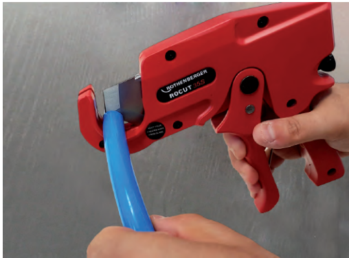
Cut the pipe with the special shear.
