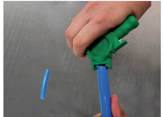
Use the calibrator tool to chamfer the pipe end and restore the correct shape after cutting.
