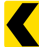
Chevron Alignment Marker
