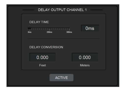
**DELAY TIME:** Adjusts the delay time of the output audio signal, measured in milliseconds.
