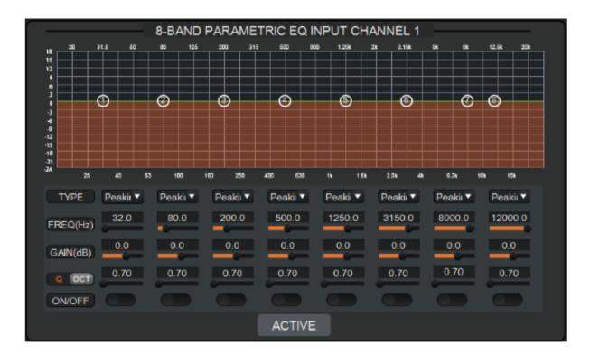
**TYPE:** Provides 5 types of band/filter, with H-Pass, L-Pass, H-Shelf, L-Shelf and Peaking optional. **FREQUENCY:** In High/Low Pass Filter, it means the cut-off frequency of the EQ band; In Peak Filter, it means the center frequency point of the EQ band; with a scale of [20, 20000] Hz.
