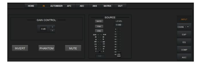
**GAIN CONTROL:** Indicates the GAIN level of the input signal, which could be adjusted to ensure the gain on the input channel adaptable to the MIC or linear input.
