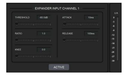
THRESHOLD: The level that the signal below it will be identified as noise and attenuated, with a range of [-60.0, 0.0] dB.
