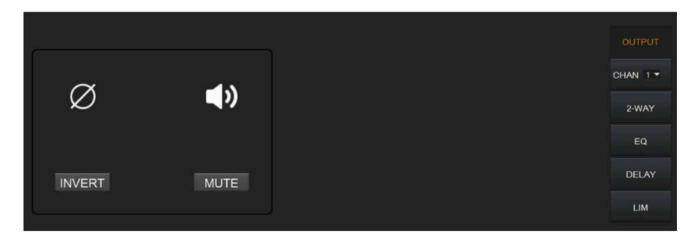
**INVERT:** When pressed, inverts the polarity of the signal on the channel.
