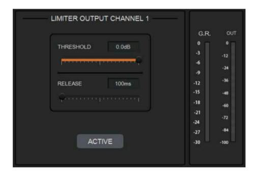
**THRESHOLD:** Shows that level signals above threshold will be attenuated, with a scale of [-60.0, 0.0] dB.
