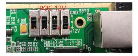
Set POC to 24V: Have the DIP switch A & C down, and the B & D to up position.
