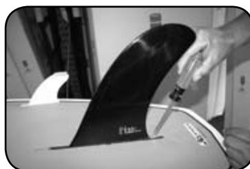
STEP 8 insert screw into fin and screw base and tighten.
