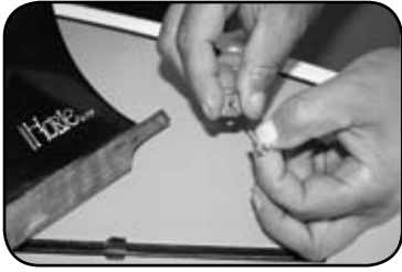
STEP 1 Remove fin screw and screw base from fin
