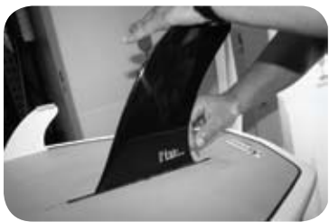
STEP 7 Line up the hole in the base of the fin with the screw base inside the box
