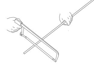
4. Now that the cover tube is cut to 10", measure the all thread tube to be 10 plus 2" long (12"). And place a mark, with a marker or tape.
