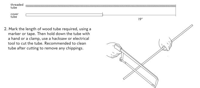
3. Now that the cover tube is cut to 15.6", measure the all thread tube to be 15.6 plus 19" long. And place a mark, with a marker or tape.
