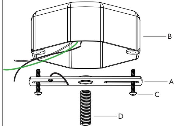
2. Cut the electrical cable to desired length and feed through the bushing in the ceiling canopy (E) and the nipple.
