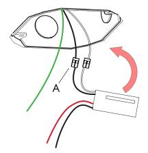
07. Bring the secondary wires and the main ground wire out from the ceiling through the center hole of the crossbar assembly. Connect a Wago Connector to wire. (B)
