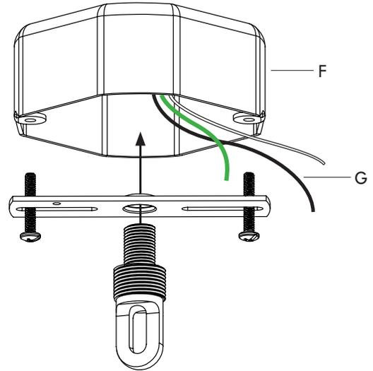
6. Carefully lift the fixture and secure the opposite hook on the stem to the hangstraight loop (H). Note that the hangstraight nut and canopy are not attached at this point and hang below the junction box connection. This will allow you to make the lead connections.
