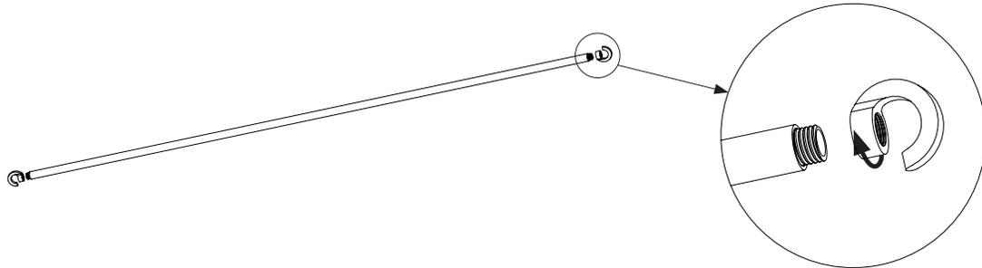
2. Attach the stem (A) to the lighting fixture (B) using the hook and loop. Feed the black lead wire (C) up from the fixture through the stem.
