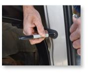
A 1/2" self-tapping screw may be added to close any gap between the Bushwacker Flare and the fender lip. This enables the Talon to securely hook onto the lip of the fender rather than the edge of the flare.
