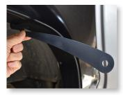
While keeping the hook attached, play with the distance between the door and the hole of the Talon. The closer the hole is to the interior face of the door, the more tension there will be on the hook. Keep in mind the door needs to be pushed towards the wheel well to release the Talon, so there is a balance between how much resistance for a secure hold vs. enough leeway in the door's movement to disengage the hook.
