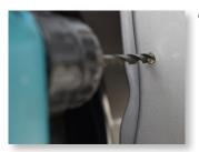
c. Use the 1/4" bit to enlarge the hole and remove any burrs.
