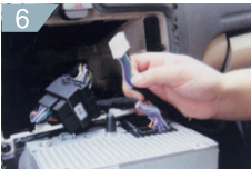
6 Pull through DSP-1 wiring harness to head unit
