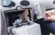
Connect DSP-1 harness to headunit wiring harness
