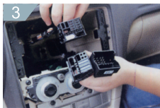
3 Install proper harness for your vehicle
