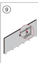
\*Attach monitor plate with M6 screws, using Allen key.
