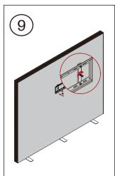
\*Attach monitor plate with M6 screws, using Allen key. Add spacers as needed.
