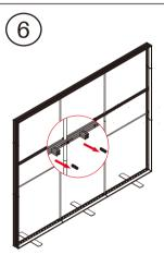
\*Remove M6 Screws from TV Bar, using Allen key.
