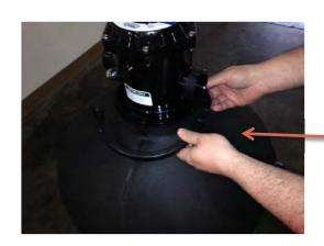
Attach Clamp using hardware provided
