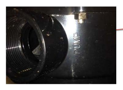
Align Valve to proper location for PUMP
