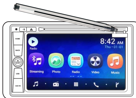
D. Use a ball point pen to push the card all the way in until it locks. Close SD slot cover.
