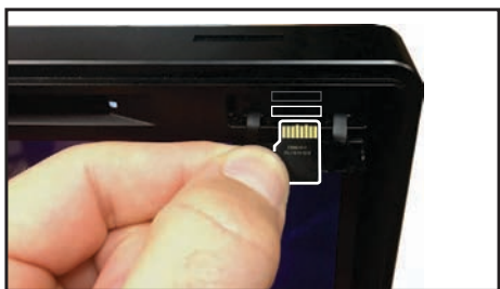
C. Insert the navigation SD card into the lower SD slot. The card inserts with the copper terminals facing up.
