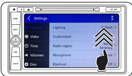
D. Swipe the right side of the screen from bottom to top to expose Navigation Hardkey Shortcut .
