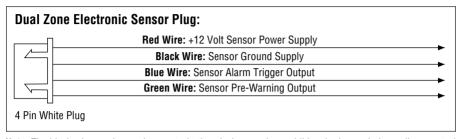
**Note:** The black wire can be used to control other devices such as additional relays, window roll up control modules or additional LED indicators. The black wire's electrical capacity is 500mA. The black wire is grounded when the alarm is armed only.
