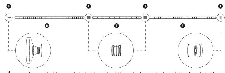
1. Install threaded inserts into both ends of the middle posts. Install the feet into the lower posts and top cap into the upper posts. Connect the upper and lower posts to the middle posts.
