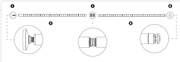
1. Install feet into lower posts, top caps into upper posts and join the upper and lower posts with the threaded inserts.
