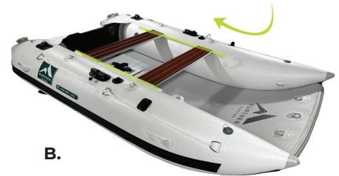
\*To improve the ease of sliding in the seats reduce the air pressure slightly in the tubes & pull the tubes together by aid of the ropes and handles.
