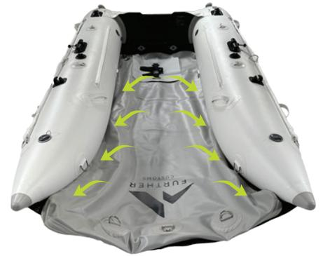
\*Note that the floor should be tucked in completely under the radius of the tubes to ensure an even floor and that the boats width is fully extended. There should be a 2-3 inch gap between the edge of the floor & transom.
