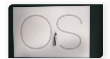
Grooving the mounting board with drill carving rotary knife
