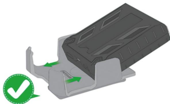
**NOTE** To Place the case face up will damage the holster.
