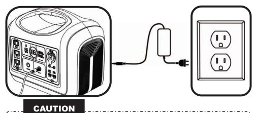
Please use our standard solar panels and adapters to charge the device, otherwise the device may not charge normally. In severe cases, the lifespan will be reduced, and the device may be damaged due to a short circuit.
