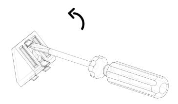
The assembly instructions will show the bottom break tab symbol on the appropriate steps where tabs need ot be broken off.
