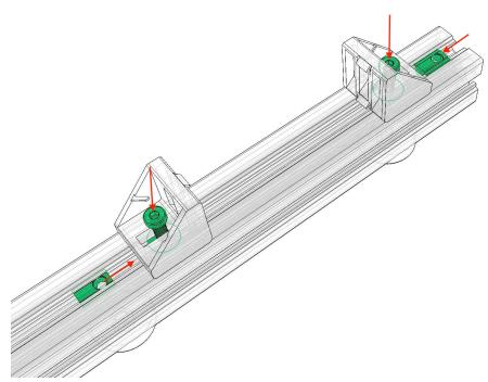
Attach the monitor stand uprights to the feet using bracket on both sides of the Upright. Make sure that the brackets are flush against all profiles.
