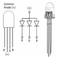
through it. The Pro Micro provides the ground signal internally (Atmega 32U4 chip) by switching a transistor on (electronic switch) based on instructions from your RGB LED sketch, providing a ground path, an internal connection to a ground pin (GND). This allows your RGB LED to light up!
