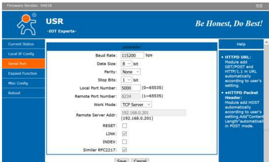
Setting Serial interface of the converter: TCP-Server mode, Port-No=5000
