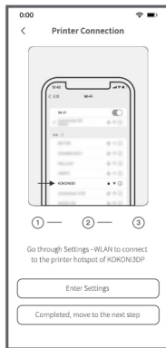
3. Printer hotspot connection: Go through Settings - WLAN to connect to the printer hotspot of KOKONI3D/P.
