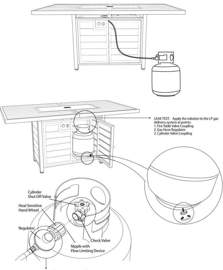
LEAK TEST: Apply the solution to the LP gas delivery system at points. Fire Table valve coupling; gas hose regulator & cylinder coupling.
