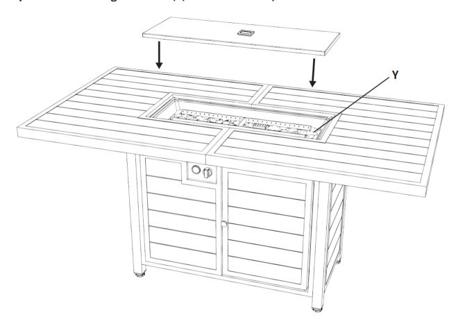
NOTE: To meet the CSA standard requirement, the burner tube must be exposed, pls don't cover the surface completely with glass stone. So we provide 10 lbs of glass stone.
