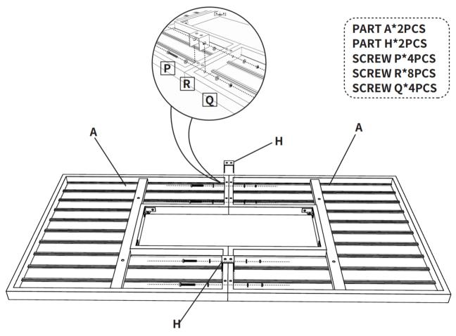
Step 2 Fix the clips (H) to frames (A) with 4pcs M6\*12 screws (T).
