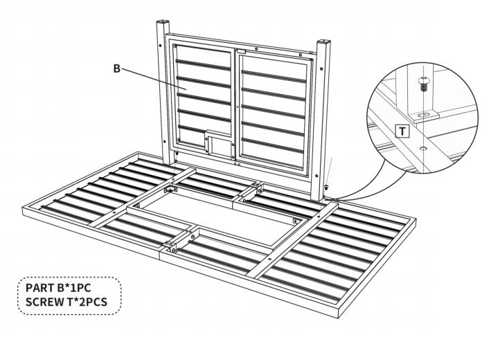
Step 4 Connect the frame(C) to the tabletop with 2 PCS screws (T).
