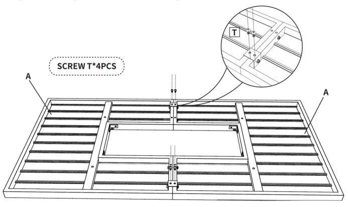
Step 3 Connect the frame(B) to the tabletop with 2 PCS screws (T).
