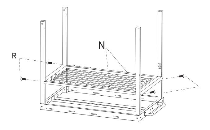
Step 7 Assemble the bottom plate E to the legs with 4pcs screw R.
