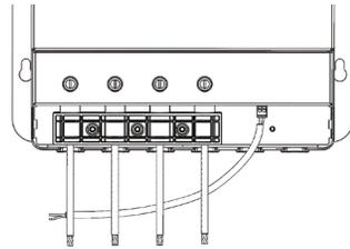
Secure the Temperature Sensor lug to one of the battery posts
