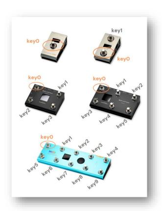
The image shows the key0 and other key numbering mapping rules for different versions of controllers. MIDI Captain series controllers with 1, 2, 4, 6, 10 switches all use the same method to enter USB configuration mode, that is **by holding down the key0**
