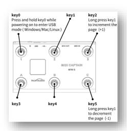
It is important to note that since the long-press page switching function of the rightmost button is fixed, please do not configure long-press and long-press release
