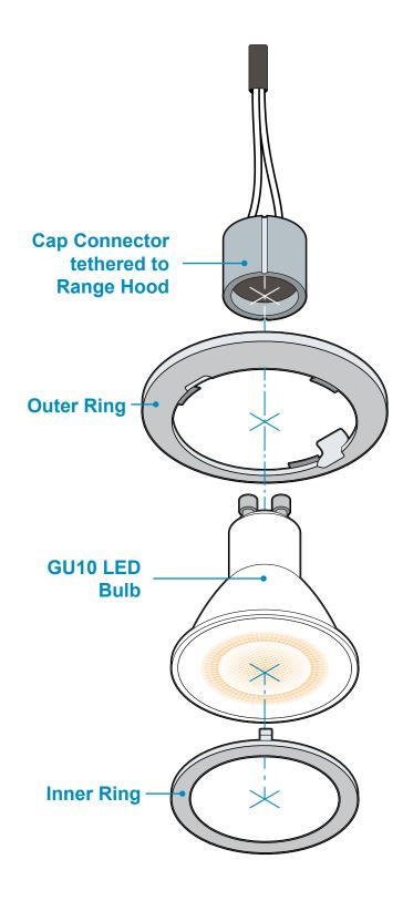
To re-assemble, simply reverse the steps (6) to (2). To re-install, (7) press the bulb housing carefully and firmly into the recess, until you hear a positive snap.
