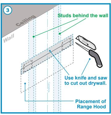
(3) Use knife and saw to cut out drywall to accommodate plywood brace support. The inserted plywood should be the same depth as the drywall slab it is replacing.
