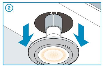
(1) Use a thin laminate card (like a business card, or plastic palette knife to preduct scratches on the metal finish) and insert in between the switch panel and LED bulb housing. Work your way around (2) until the light housing pops out.
