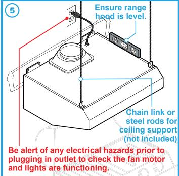
(5) Use either chain link or steel rods for ceiling support (heavy-duty, aircraft grade strength). Sold separately. Ensure range hood is level.
