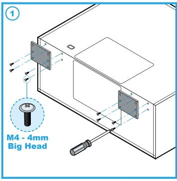
(1) Screw installation plates on to the back of the range hood.
