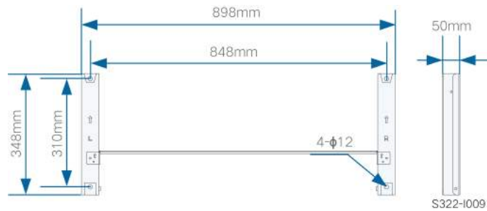
figure 4-1 Dimensions of Mounting-bracket
