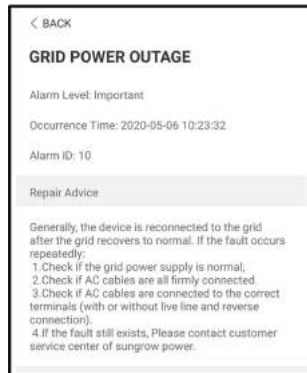
figure 7-9 Detailed Fault Alarm Information
