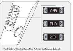
pressed to choose a mode. Then the screen will show desired temperature and current temperature. The temp LED will remain red while the pen is heating up. Once it has reached temp it will change to Green. Then you can draw. You can adjust the temperature at any time, but to change from ABS to PLA un-plug the pen and plug it back in.
