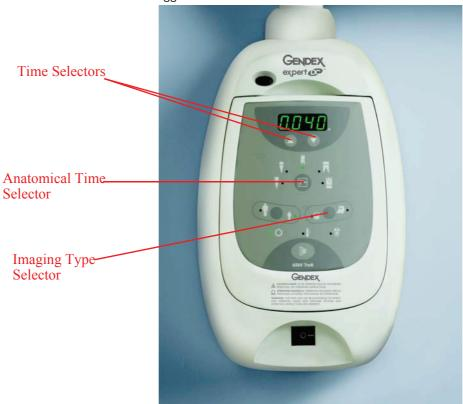
2. Press the time up or time down arrows until the LED displays SP3. The SP3 setting confirms that the system is now set for F-speed film.
