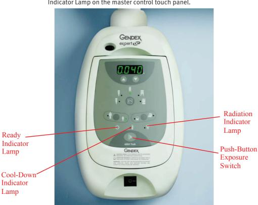
is being emitted, a yellow indicator light appears next to the Radiation Indicator Lamp on the master control touch panel.
