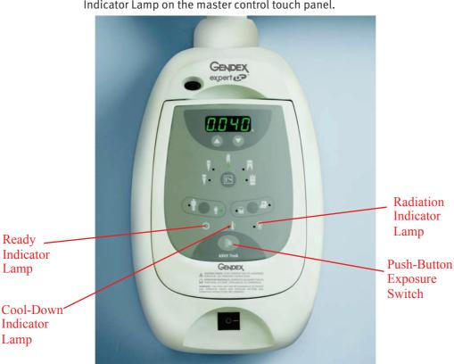
is being emitted, a yellow indicator light appears next to the Radiation Indicator Lamp on the master control touch panel.
