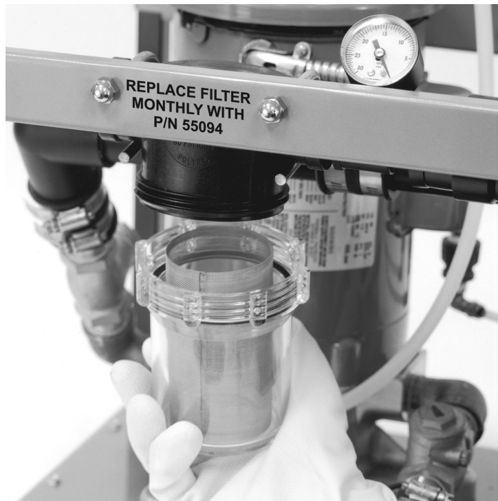
Figure 12. Intake Solids Collector Location
