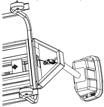
16. Connect the handle using the 4 x M5 x 30 screws provided.
