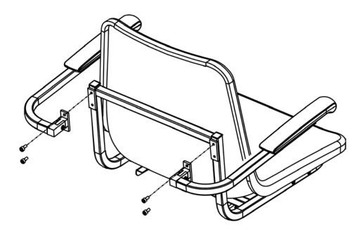
18. Place the chair assembly onto the base and secure using the 4 x M5 x 15 screws provided.
