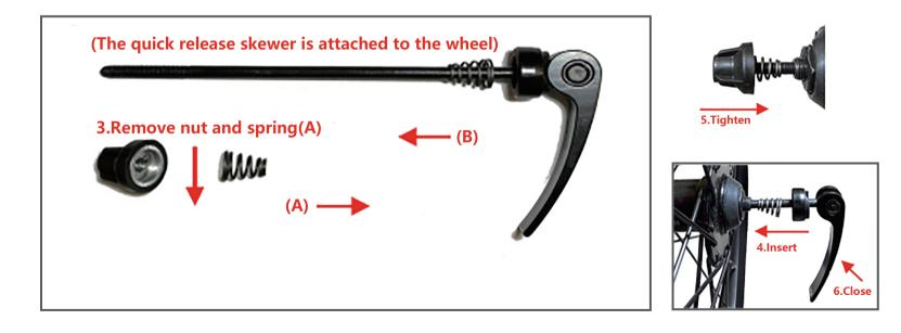
(C)Rear Wheel (required tools: 18mm wrench, recommended torque 40 N.m)
