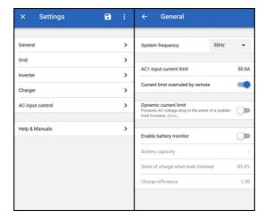
You can only access Settings with a MK3-USB. You cannot use a VE.Bus Smart Dongle to access Settings Mode.
