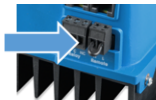
Remote connector with wire loop
