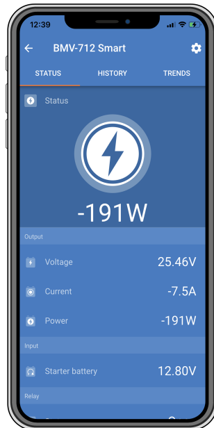
VictronConnect status screen of a battery monitor running in DC monitor mode.
