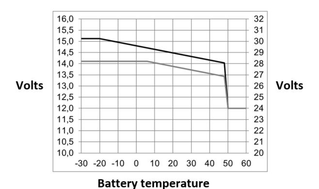
Default output voltages for Float and Absorption are at 25 °C.
