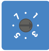
Rotary switch set to position 2
