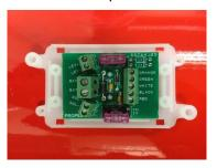
Secure the junction box provided internally in the vehicle and run the two cables from the tank to the junction box. Make the connections as indicated on the board. The White and black pair are the level sender. Bring your 12v DC feed from your leisure system into the centre block.
