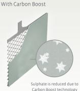
During discharge, non-conductive sulphate particles progressively cover the negative plates, isolating them from the electrolyte. This means a lot of the energy intended to recharge the battery is needed to dissolve the sulphate, which makes charging less efficient. The high-surfaced carbon additives in Fulmen's Formula Xtreme Carbon Boost battery provide superior conductivity, dissolving the sulphate particles
