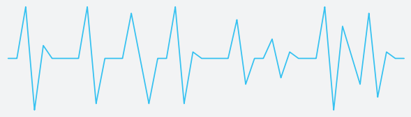
Typical pattern of State of Charge during a journey with Start-Stop system
