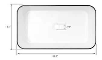
The values indicated on the drawing are theoretical product dimensions. A permissible deviation of 0.4 in. is allowed for appearance dimensions. Please refer to the physical object for accurate measurements.
