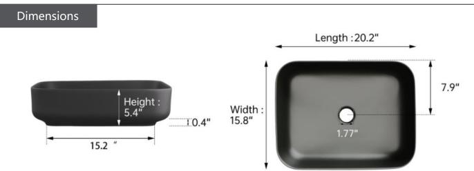
The values indicated on the drawing are theoretical product dimensions. A permissible deviation of 0.4 in. is allowed for appearance dimensions. Please refer to the physical object for accurate measurements.
