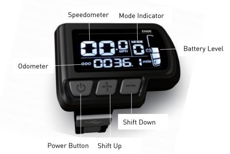
Speedometer: Display the speed of the ebike Mode Indicator: Display Mode1/Mode2/Mode3 Odometer: Shows the total mileage of the ebike Battery Level: Each icon means 20% of battery level Shift Up/Shift Down:Shift power mode between Mode1/ Mode2/Mode3 Power Button:Hold the button to power on/power off
