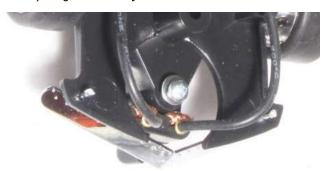
The lower front spoiler attached to the chassis with two vertical pins. When the cement dries cut the two pins flush with the top of the chassis so they do not interfere with the body mounting.
