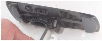
Use a square jewelers file to enlarge the hole in the interior to accept the square pin on the bottom of the driver's head.
