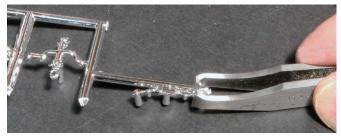
You can avoid damaging the smaller plastic parts by cutting them from the sprue with special flush-cut diagonal cutters (called "sprue cutters") designed for use by modelers.
