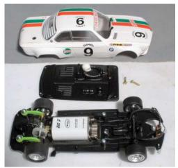
Test-fit the body and the interior. I had to trim the inside of the nose about 1/32-inch to clear the front of the chassis. Assemble the interior and body on the chassis and test run the car.
