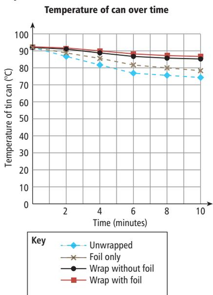
1. No covering. The can without any insulation allowed the water to decrease in temperature most in 10 minutes.
